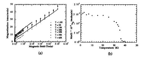
FIGURE 1. a) Magnetisation versus applied field for a series of temperatures. Solid lines are least squares fits to the linear region of the data. b) Zero field extrapolated magnetisation as a function of temperature.
