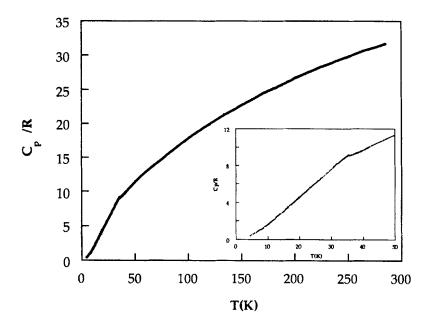
FIGURE 2. Heat-capacity of  $1\beta$ . The inset magnifies the anomaly observed at 35.5K
